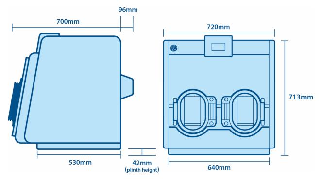
**Important note:** In addition to the dimensions stated above, allow a localised protrusion of 90mm at rear to accommodate condenser bottle, bracket, gas and electrical supplies. If bench mounted, a further minimum clearance of 500mm is required above the unit and a minimum clearance of 500mm at the right-hand side of the unit is required for user/service access.
